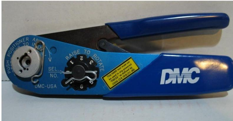
AFM8 Positioner for Standard D-Sub Connectors
