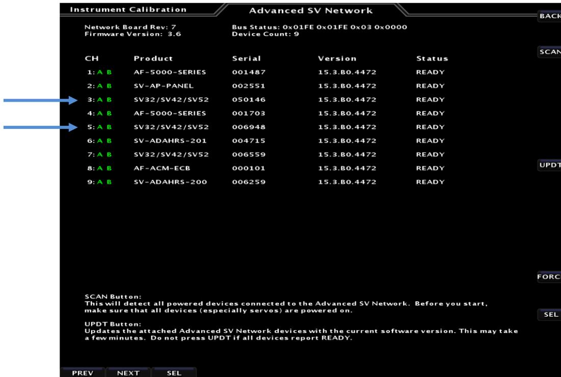
2. Perform the **3. Servo Calibration** and **4. Servo Test** following the PFD EFIS on screen directions. After completing these steps both items **MUST** show **COMPLETE** before the Autopilot can be used. The following settings are from a Van's RV-14 and RV-10.
