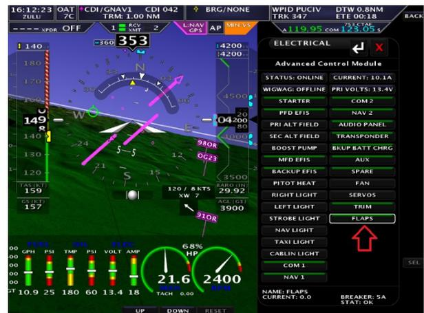
**10. Endpoint Slop Timeout** The Flap Motor will continue to run for this number of seconds to make sure the flaps are fully retracted or extended. The flap positioning system should not be used to provide an accurate position stop for full flap up or down settings.
