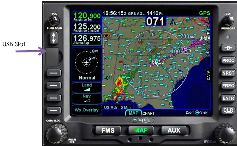
To enter configuration mode you will need to power up the IFD with a USB memory stick.
