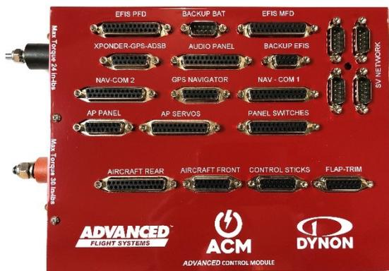
**ACM module with Electronic Circuit Breakers**
