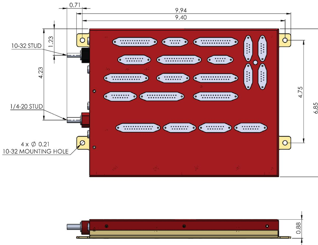
**Do not over-torque the power terminal nuts, they are soft copper and will break if over-torqued.**
